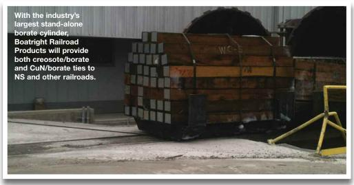
stranger to innovation, Boatright Railroad Products owns the first wood-preserving plant to produce creosote/borate dualtreated ties on a commercial scale.
